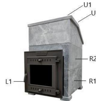
1. The side walls shall be installed starting from the 1st level from the portal extension hole clockwise. The assembly shall start with the installation of the hole supports B1 and the block part number L1, then in numerical order (F1, R1). The parts are connected to each other using the fasteners between the rows and blocks. All parts of the soapstone are marked to indicate the level and the direction.
