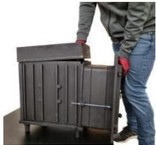
4. Apply a heat-resistant sealant to the grooves in the front wall (11c). Place the front wall with the lower edge on the base of the stove, lift the front edge of the stone tray, press the front wall firmly against the edges of the side walls and lower the stone tray.
