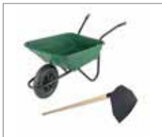
Wheelbarrow / Hoe (mortar preparation)
