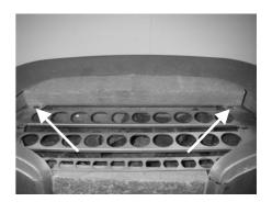
Install the round-edged stone next. Push the other end under the edge and then push the stone along the support plate against the end limiter.
