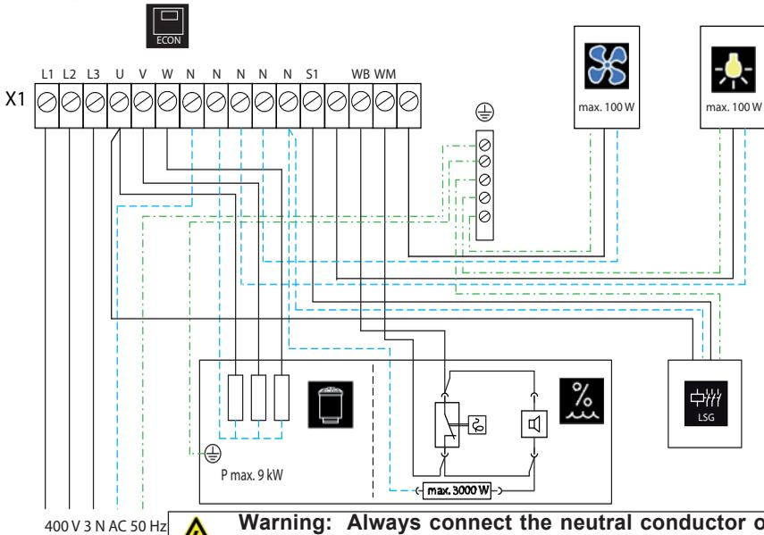
**Warning:** Always connect the neutral conductor of the sauna oven. During steam operation, one phase of the oven is shut down; therefore the heating load is no longer symmetrical. The result is that the neutral wire is no longer current-free.
