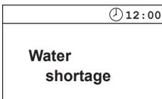
If no water is refilled the system switches off after 2 minutes.
