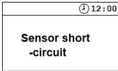
= Short-circuit in the room sensor circuit
