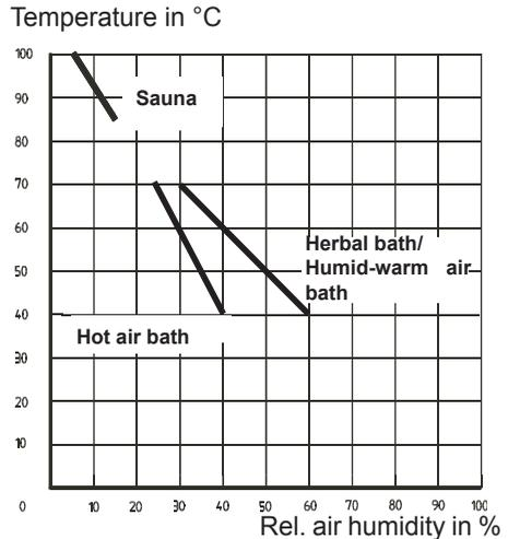
The humidity intensity shown in the display corresponds to the time proportional evaporator setting. Therefore, the relative air humidity is not preselected or shown on the display, but rather the switch-on frequency of the evaporator in percent. The graphic is intended to clarify this.
