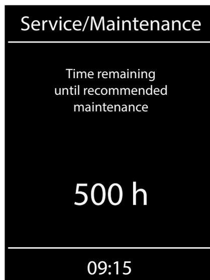
The amount of time remaining until the next service date is displayed. The operation time is set to 500 hours by the factory.
